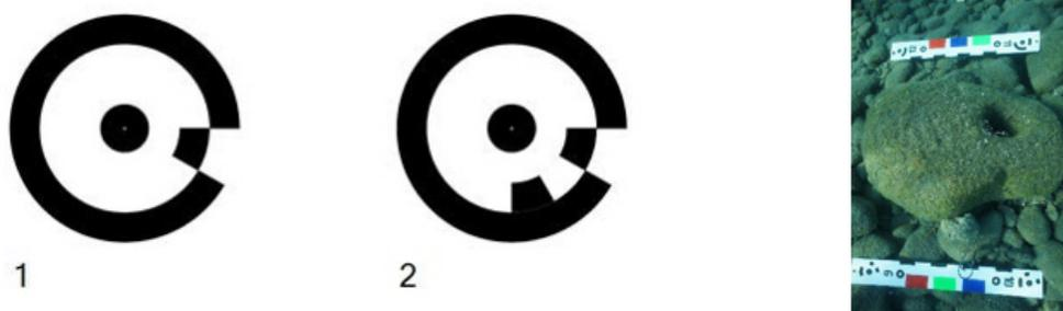
Figure 9: Coded targets used in conjunction with length and colour scale (Wreck Check Inc.)
